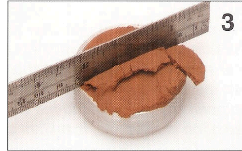
3. Remove excess clay with a ruler. Turn the clay filled upside down.
